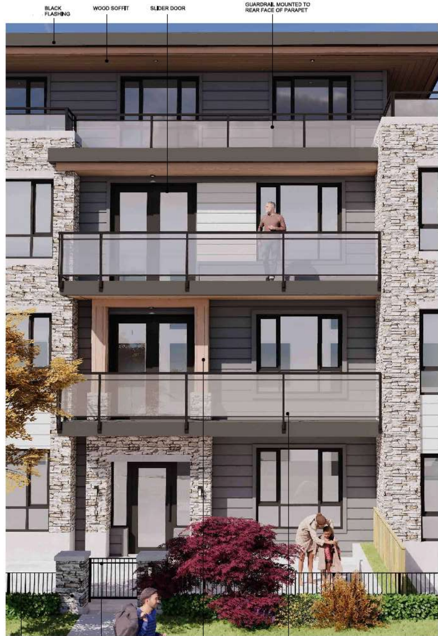
GATE POST STONE PORTICO POST AROUND GROUND LEVEL HEAVY TIMBER POST FRAMING LEVEL 2 BALCONY DOOR GUARDRAIL MOUNTED TO FRONT FACE OF FACIA
