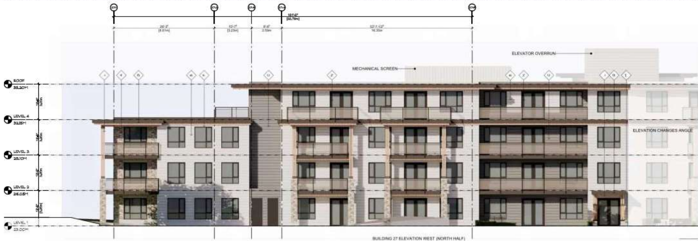
BUILDING 27 ELEVATION WEST (NORTH HALF)
