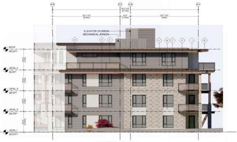
2. BUILDING 27 ELEVATION NORTH
