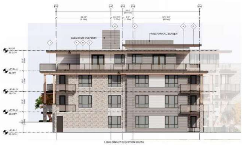
1. BUILDING 27 ELEVATION SOUTH
