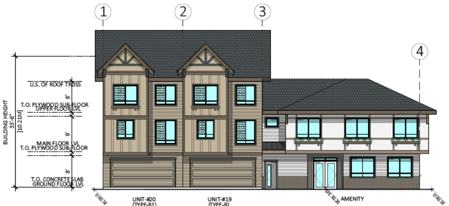
1 ELEVATION AT GARAGE SIDE FACING (NORTH) 1/16"=1'-0"
